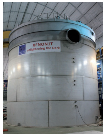
Fig. 3: Water tank for XENONnT installed in hall B of LNGS.
